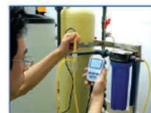
Cond./Res. Measurement of high purity water
